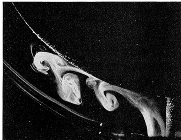
Fig. 2 Tracer element enters annulus with incoming fluid, Re = 411
